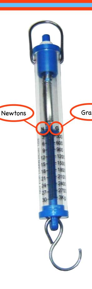
This is a FORCEMETER. Forcemeters are used to measure forces. Forces are measured in newtons. Some forcemeters also have readings in grams as they convert the force to a weight. Forcemeters have a hook at the bottom to attach to the object being measured and a spring inside. The spring stretches as the force is applied to the hook. The reading can then be taken where the spring stops to see what the force measurement is.
